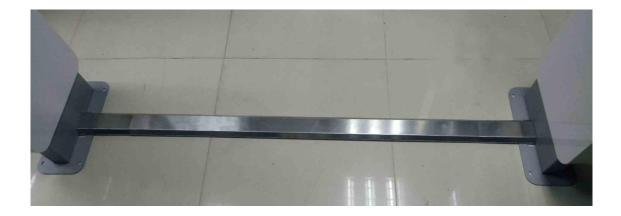
The trunking cover is made of 1.2MM stainless steel and can withstand an external weight of 100 KG.
