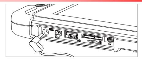
When the AC Adapter is connected, the battery pack starts charging. The battery LED indicator on the tablet computer will show different states. Please refer to description of the LED indicator in the Description of Parts.
